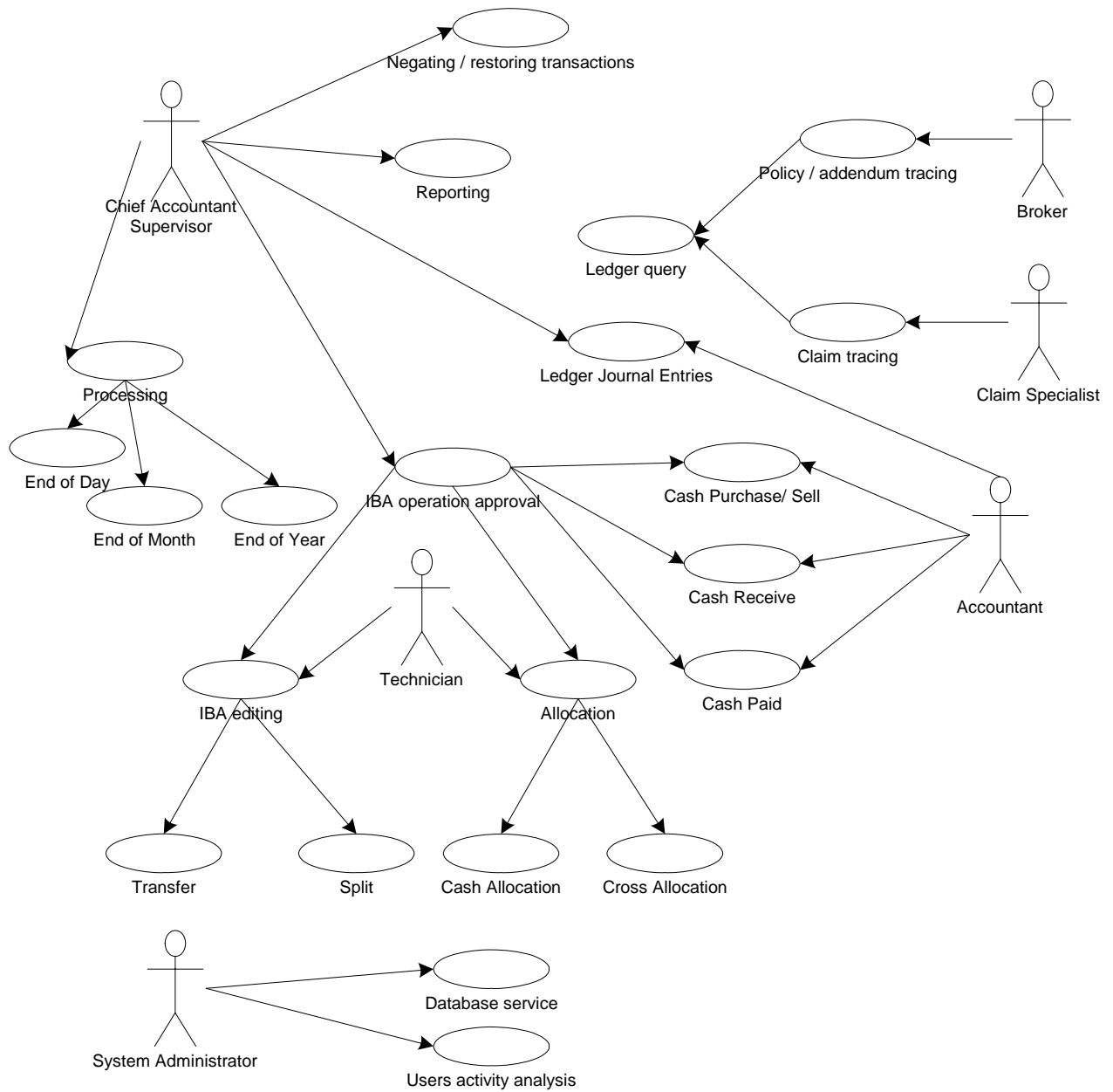
Figure 9. Use Case Diagram
